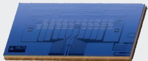
**Figure 1.** Biosensor based on photonic integrated circuits.
